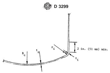
FIG. X2.1 Thickness of Dished-Bottom Head
