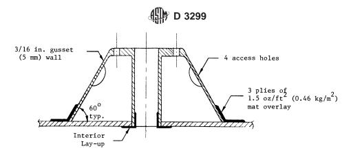
NOTE 1—This design does not require lay-up of nozzle neck to exterior of tank wall. Nozzle may be penetrating type or flush type as illustrated. FIG. 5 Conical Type Gussets
