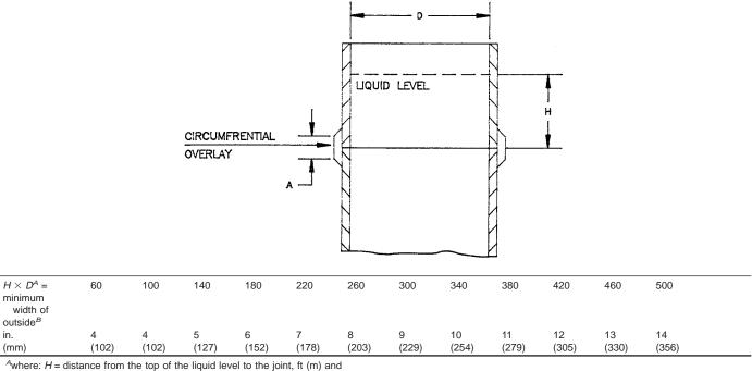
TABLE 3 Minimum Widths of Joint Overlay for Circumferential Joints
