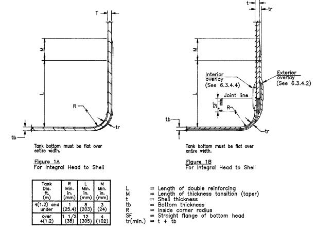
FIG. 3 Flat-Bottom Tank Corner Detail
