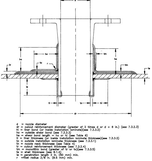
FIG. 2 Penetrating Nozzle Installation
