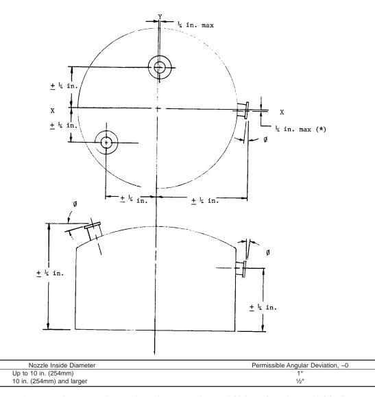
Note 1—Larger tolerances may be agreed upon between purchaser and fabricator for tanks over 12 ft in diameter. FIG. 8 Nozzle Location and Orientation Tolerances
